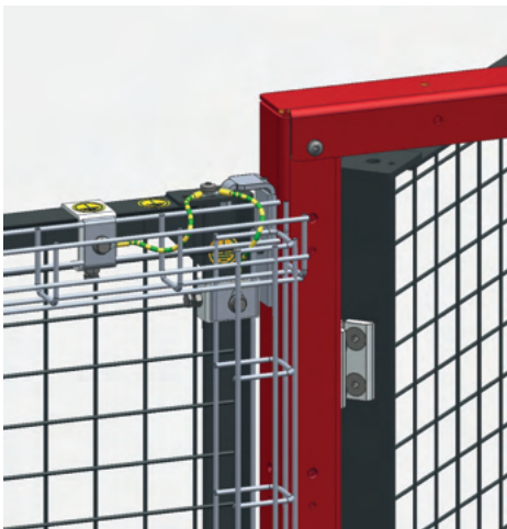
Example of earthing the cable ducts
